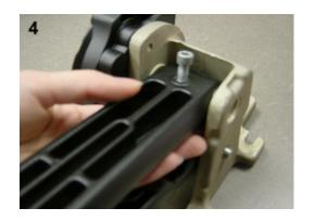
Unscrew 1/4-20x7/8" Socket head or Hex cap screw located at the top of the **rear** linkage arm 3 to 4 turns and strike head of bolt with a hammer lightly to push wedge loose of linkage. The front linkage arm has the AMP Research logo attached.
