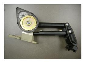
Install New Clutch-Gear assembly or Drive shaft thru bushings in the upper mount.
