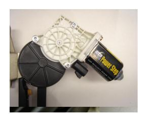
Move board by hand so motor/gear box assembly drive gear will engage with shaft and bolt holes will align.
