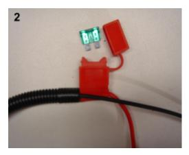
Remove fuse from the AMP wire harness. Fuse is located 6-8 inches from positive battery terminal.
