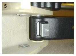
Remove aluminum wedge. Make note of the threaded hole orientation.
