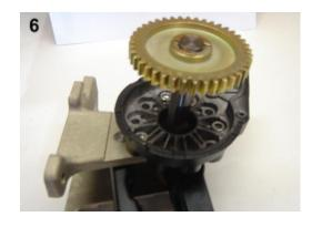
Slide out **clutch-gear assembly** shown if using (3) bolt motor or remove the Drive shaft if using a (2) bolt inline motor.
