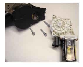
Unplug motor and remove (3) socket cap screws with motor shown or (2) bolts with inline Bosch motor and remove entire motor/gear box assembly from linkage.
