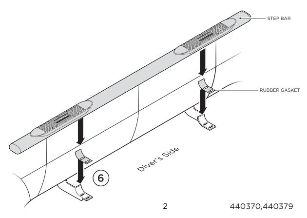
**7.** Attach the Step Bar onto each Bracket using two (2) M10 x 30MM Button Head Bolts, two (2) M10 Flat Washers and two (2) M10 Lock Washers per bracket.
