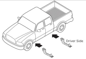
**4.** Insert one (1) M10 Bolt Plate into the hole on the Rocker Panel. Make sure the Plastic Push nut is on the stud of the Bolt Plate to hold it into place.
