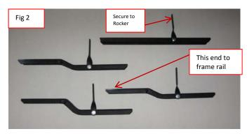
**Step 4:** Measure and mark the suggested mounting locations of main brackets on pinch weld of vehicle. From the Front wheel well measure the following: 12", 26.5", 43" and 57.5".
