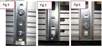
There are several configurations to mount the boards to the brackets. We have provided some suggestions in the figures above. These changes allow you to adjust the board in or out according to your step preference. All are correct.
