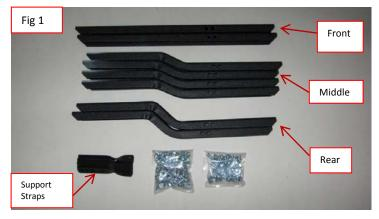
**Step 2:** Separate and identify the brackets (one front, two middle brackets and one rear bracket for each side of the vehicle.
