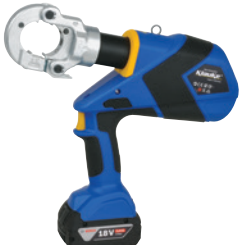
EK 60/22 BATTERY-POWERED HYDRAULIC CRIMPING TOOL 6 – 300 MM², BOSCH BATTERY 5 AH Large crimping range up to 300 mm². Fast crimp cycles due to Automatic Retraction Stop (ARS). Suitable for 22-series interchangeable crimping dies, narrow crimping.
