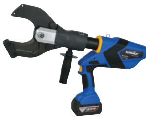
ES 85 BATTERY POWERED HYDRAULIC CUTTING TOOL 85 MM DIA. , BOSCH BATTERY 5 AH Cuts copper and aluminium cables with lightweight steel armouring (depending on cable type). Large cutting area. Also suitable for fine-stranded cables (depending on cable type).
