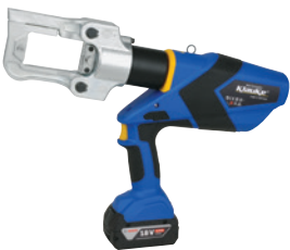
EK 120 UNV BATTERY-POWERED HYDRAULIC UNIVERSAL TOOL 10 – 400 MM², BOSCH BATTERY 5 A One head for crimping, cutting and punching – one tool for all. Ideal in the assembly field where all common jobs can be carried out using one tool.
