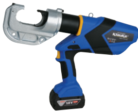
EK 120/42 BATTERY POWERED HYDRAULIC CRIMPING TOOL 16 – 400 MM², BOSCH BATTERY 5 AH C-head with very wide crimping range to 400 mm². Up to 60% fewer crimps thanks to wide crimping in comparison to 6 t tools. Easy handling by optimum weight distribution. Suitable for 13-series interchangeable crimping dies, wide crimping. Open head, rotatable.
