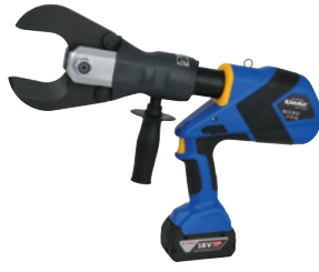
ES 65 BATTERY POWERED HYDRAULIC CUTTING TOOL 65 MM DIA. , BOSCH BATTERY 5 AH Cuts copper and aluminium cables with lightweight steel armouring (depending on cable type). Also suitable for fine-stranded cables (depend-ing on cable type). Extremely robust design with low weight.
