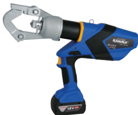
EK 120 ID BATTERY POWERED HYDRAULIC CRIMPING TOOL 35 – 500 MM², BOSCH BATTERY 5 AH Indent crimping for superfine-stranded conductors up to 500 mm². Universally applicable without changing dies, no crimping dies required.
