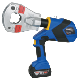
EK 60 VP/FT BATTERY POW-ERED HYDRAULIC CRIMPING TOOL 16 – 300 MM², BOSCH BATTERY 5 AH Crimps optimised at all times due to the patented centering system. Suitable for crimping tubular cable lugs and connectors “standard type” and fine and superfine stranded conductors to 300 mm².
