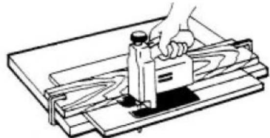
Figure 5 - Cutting AVONITE Flex Sheet with Sabber Saw
