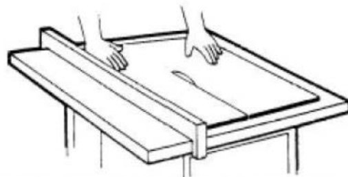
Figure 4 - Cutting AVONITE Flex Sheet on Table Saw
