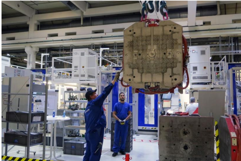
As the number of variants increases, so does the number of setup processes. To keep these efficient, all duo machines are equipped with magnetic rapid clamping systems.
