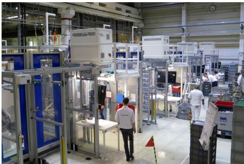
The multi-component process runs on a duo 700 combi injection moulding machine by ENGEL. The Faurecia plant in Peine currently produces various black panel components for the Audi Q8 and Q3 models on five duo machines.
