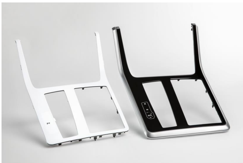
These centre consoles are made of PC-ABS and two PC grades in three-component injection moulding (left) and then high-gloss painted (right). The shift position P is backlit. For this purpose, the paint is partially removed with the aid of laser engraving.
