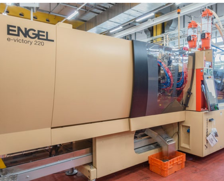
The e-victory 220 injection moulding machine is exclusively used for the production of damping cylinder housings.
