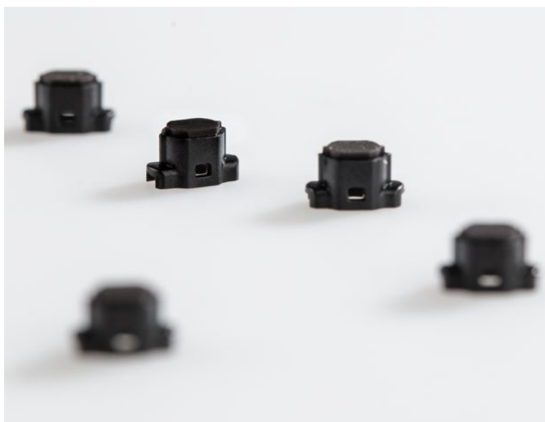
The air inlet valve is produced in a single injection moulding step from polyamide and liquid silicone rubber. The functional element is only 4 mm wide and 3 mm high.
