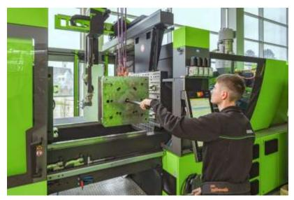
Given the right approach, a huge amount of time can be saved during mould set-up. For example, with the Setup wizard, which interactively guides the machine operator through the individual steps.
