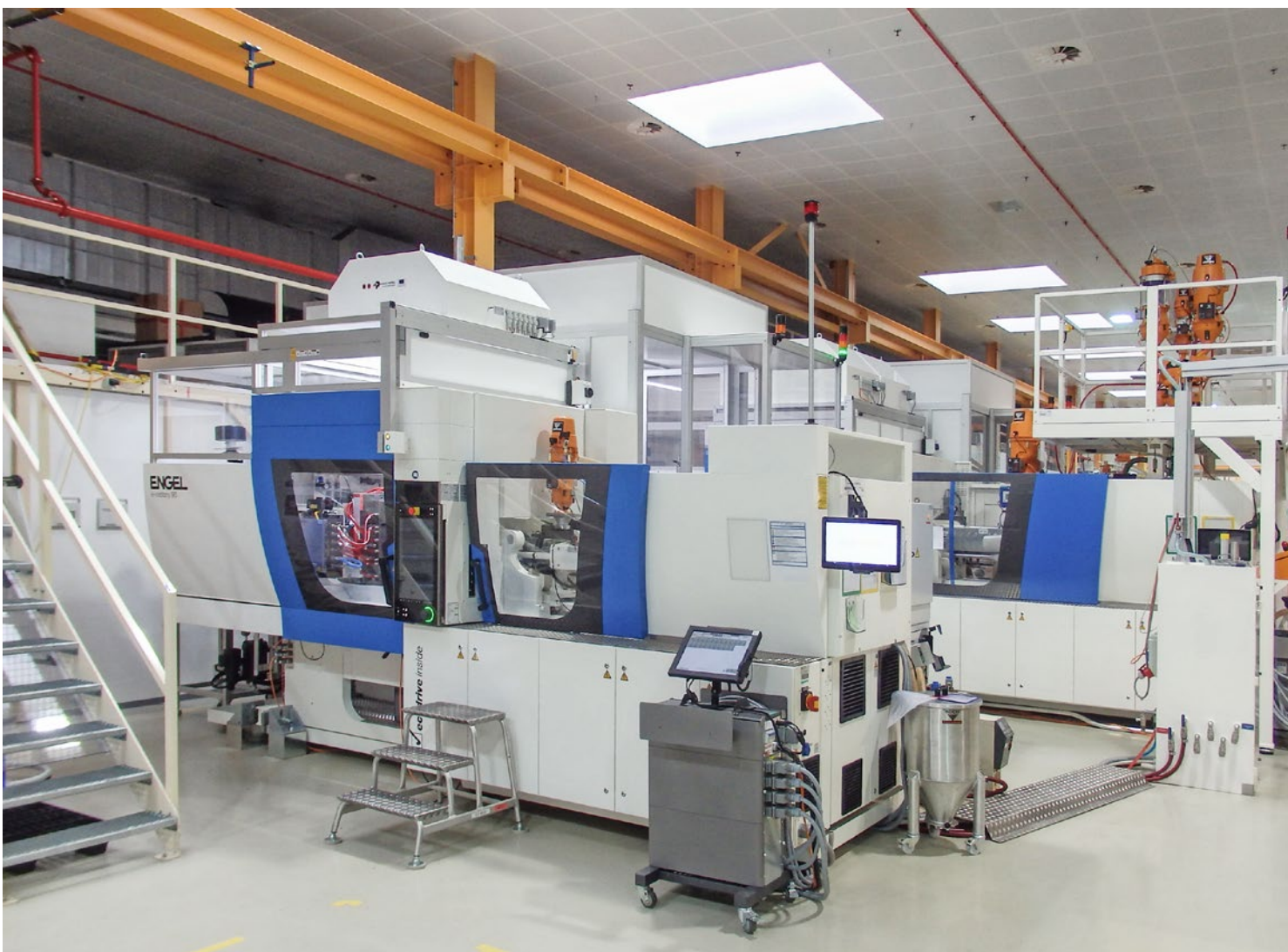
The injection moulding machines and automation are encapsulated in clean-room-compatible production cells in compliance with ISO 7 requirements.
