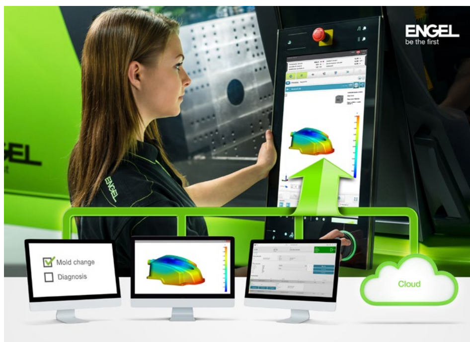
The WebViewer tool on the machine control unit integrates auxiliaries with web interfaces as well as data from internal and external systems that is accessible via a browser.
