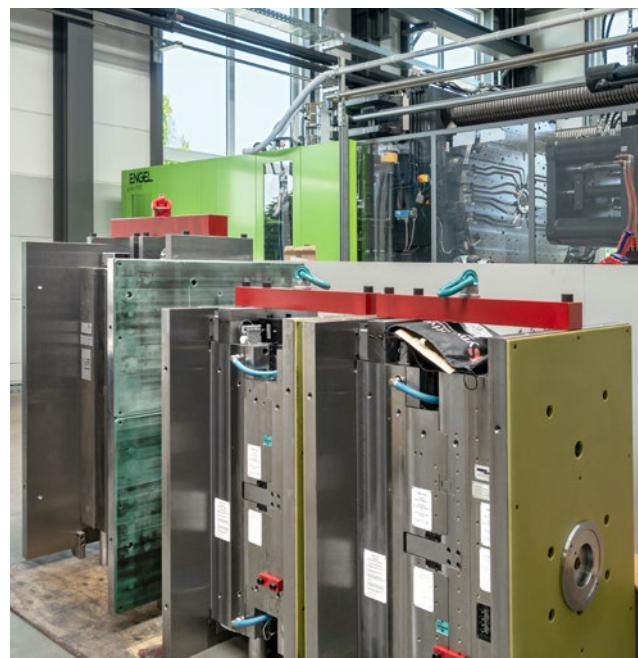
With its indexing table and rotary table, the duo combi M is ideally equipped to handle all types of multi-component requirements.
