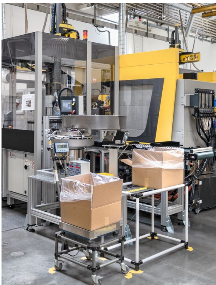
For the new production process, Interroll invested in an integrated manufacturing cell with an ENGEL victory 120 injection moulding machine and an ENGEL viper 12 linear robot.
