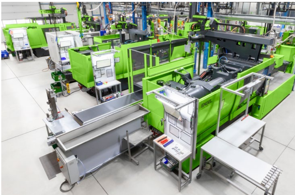
R+M/Suttner has installed nine new ENGEL victory injection moulding machines with robot and inject 4.0 technology at its Leopoldshöhe production plant.
