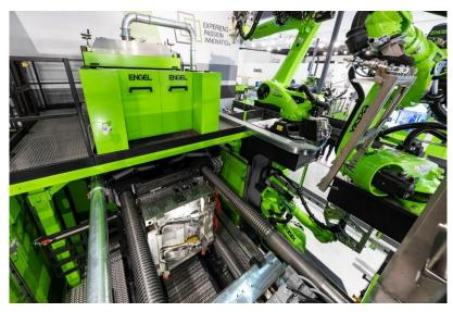
For the production of the door modules, three organic sheets of different thicknesses and shapes are heated, formed and functionalised in injection moulding in a fully automated process.
