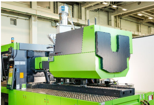
Fig. 1: The new all-electric high-performance injection units from ENGEL significantly expand the application range of electric injection moulding machines for thin-wall injection moulding.
