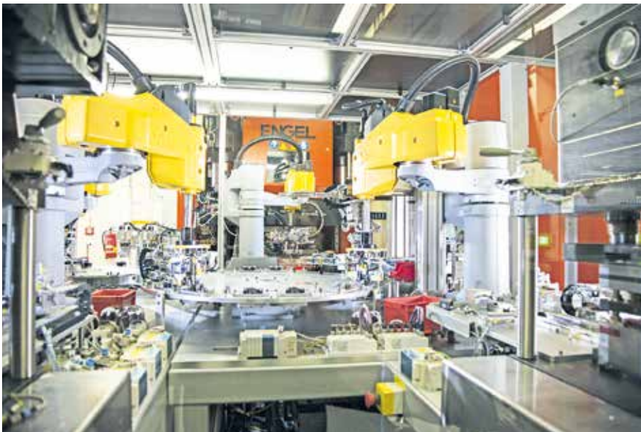
Fig. 4. Engel has expanded its easix series further with Scara robots. They are utilized for fast pick-and-place tasks, such as the efficient full equipping of grips or buffer adapters (figure: Engel)
