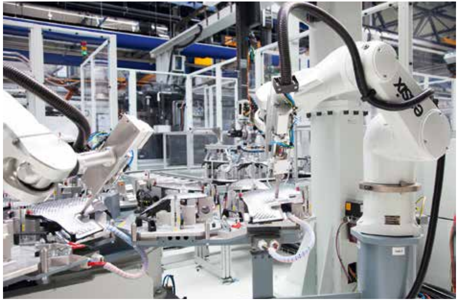
Fig. 3. The stand-alone version of the multi-axis robot – as here at Weidplas in Treuen, Germany – makes it possible for production operations to work with an integrated solution and a uniform operating logic via the injection molding process (figure: Weidplas)
