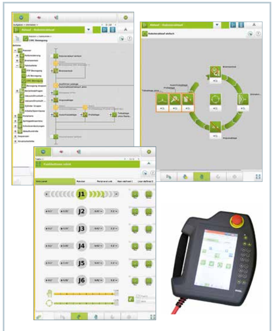
Fig. 2. Complete control integration enables simple parameterization and operation of the easix multi-axis robot. The Engel solution enables object oriented graphical representation of flow sequences even for complex production processes. Teach skills for the viper linear robot are all that is needed (figure: Engel)
