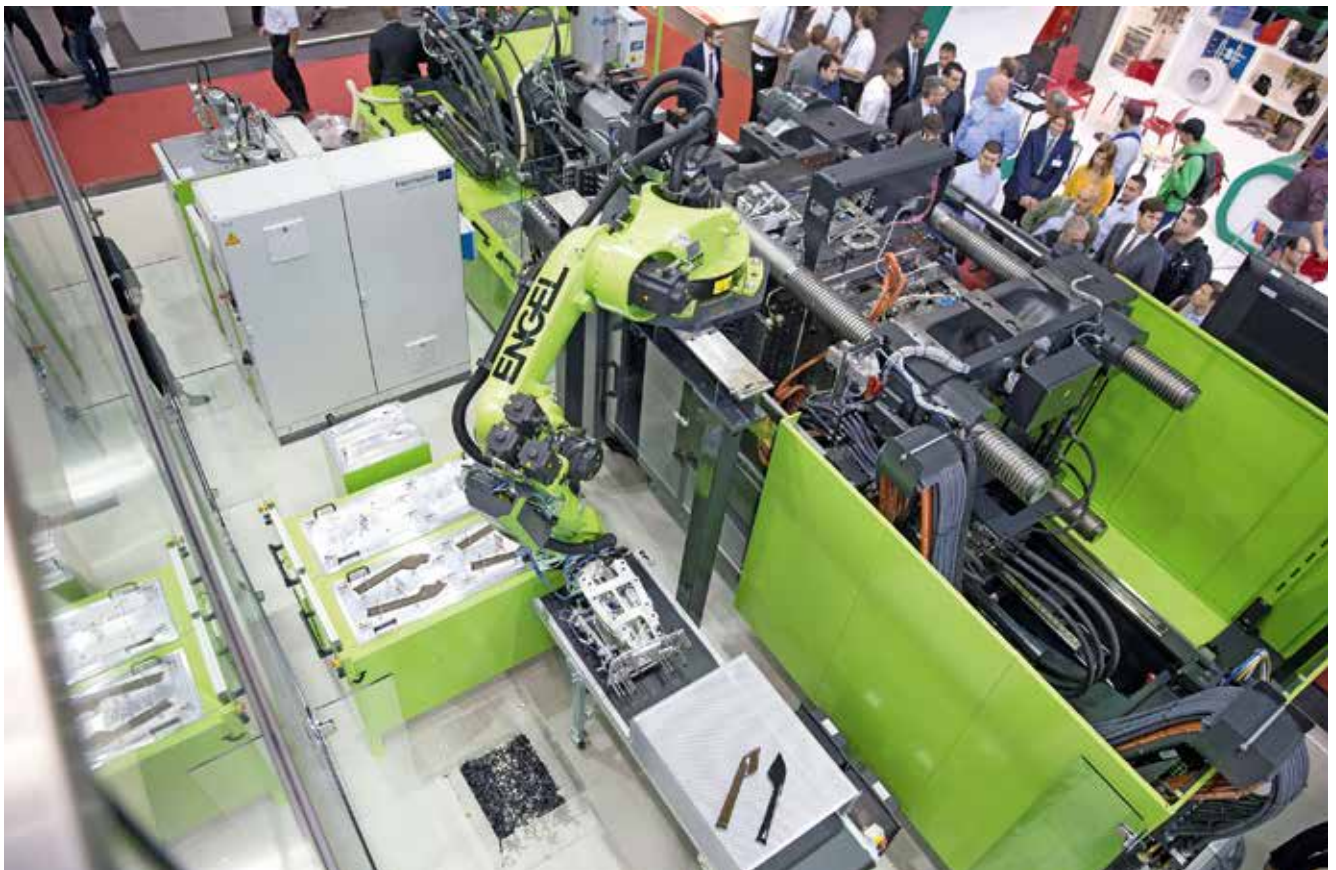
Entirely integrated: An Engel duo combi M injection molding machine produced decor elements for an automobile interior at the 2015 Fakuma. An Engel easix industrial robot performed the handling of real wood veneers and the finished parts (figure: Engel)
