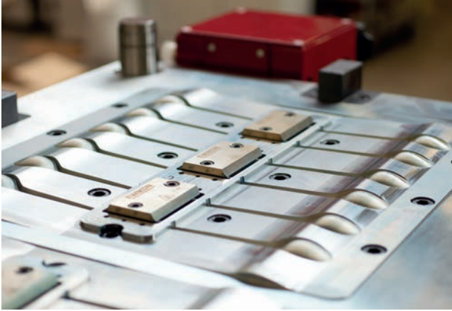
Fig. 3. Particular of the 24-cavity mold for the production of ice cream spoons. © Ewikon
