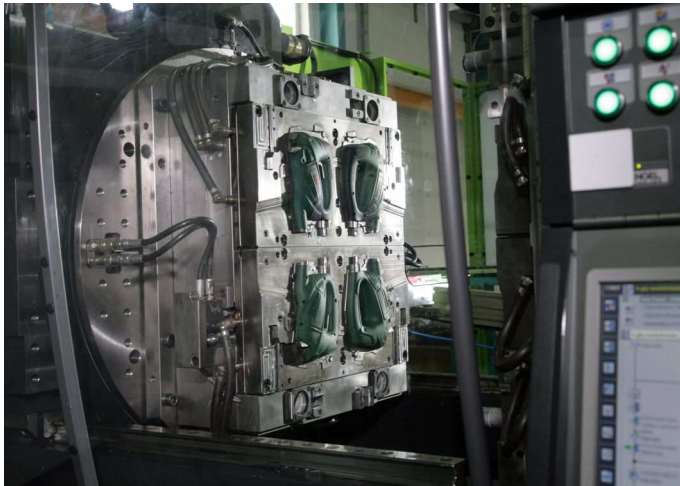
As mould fixing platens on the tie-bar-less ENGEL victory injection moulding machines can use all the space right up to the edge of the machines, large moulds fit on relatively small machines.
