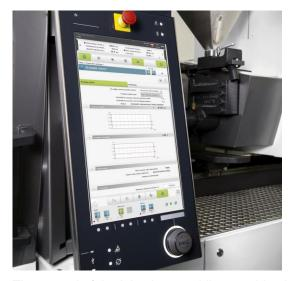
The control of the injection moulding machine is becoming increasingly intelligent. With the help of assistance systems such as iQ weight control, the injection moulding process is continuously self-regulating.
