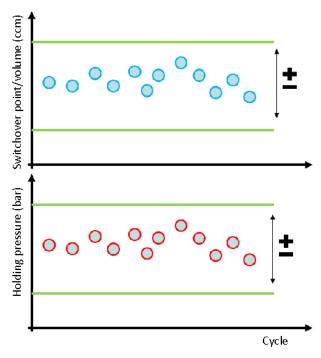
The key for the validation of processes with dynamic control lies in the definition of process windows for the adjustable process parameters.
