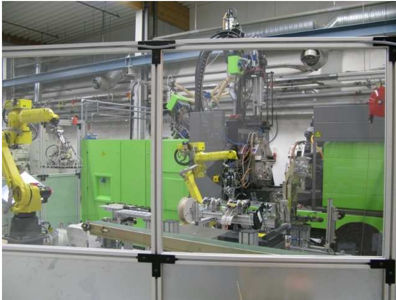
The production cell for manufacturing the OneLED lamps works autarchically on a minimal footprint. (Fig.: Hella)
