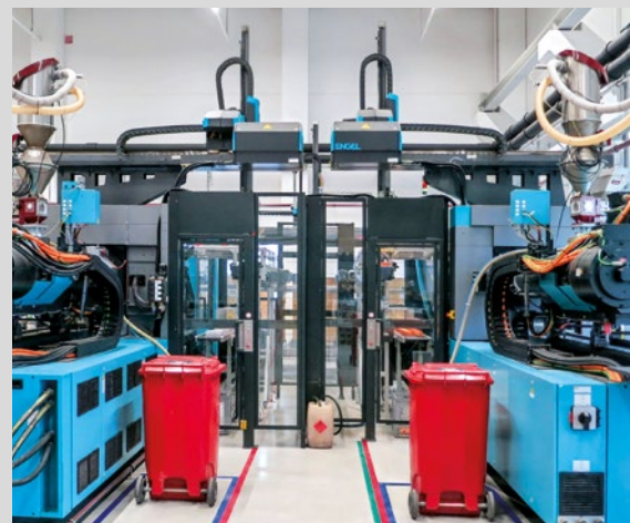
The container caps – both round and square – are produced on two adjacent e-motion machines, which are also equipped with viper robots.
