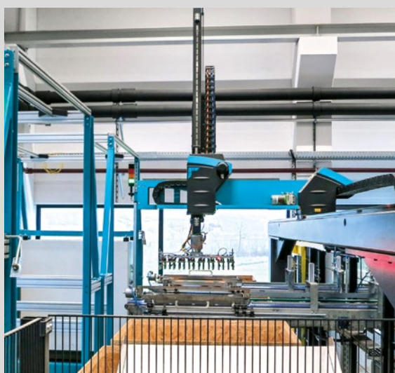
ENGEL viper stand-alone version: In combination with the transverse carriage (on the left in the photo), the robot connects the injection moulding production with the high-bay warehouse. Every ten seconds the viper robot reports the current quantities to the warehouse.
