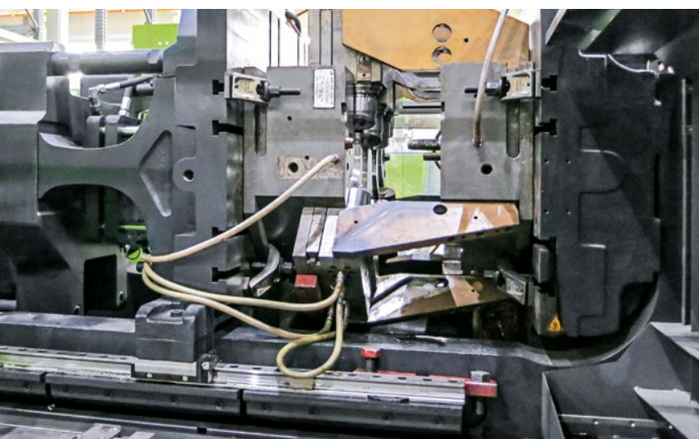
Even with complex moulds, the clamping force required for the moulding process and not the mould dimensions determines the size of the injection moulding machine used.
