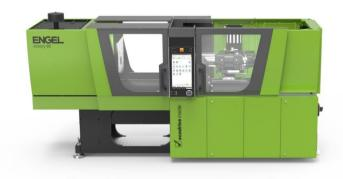
With their tie-bar-less clamping units, ENGEL victory injection moulding machines combine high production efficiency with consistently high component quality.
