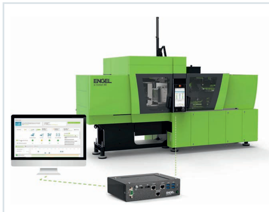
Fig. 4. The algorithms of the assistant run outside the machine on the Edge Device. The external computer also supplies data to web applications if required, and thus acts as a gateway to the world of digitalization © Engel
