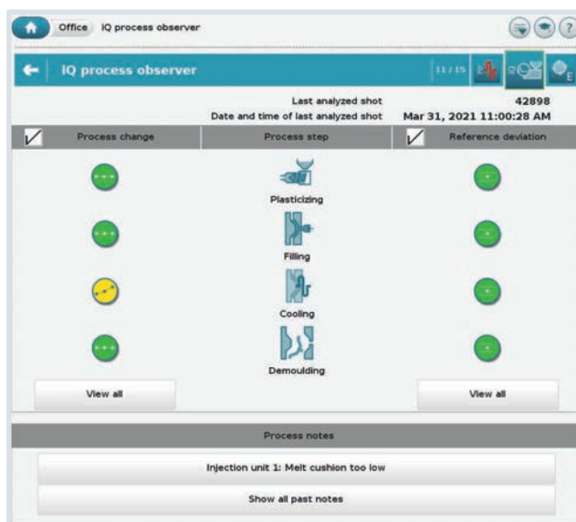
Fig. 1. The overview page of the iQ process observer summarizes all the information about the current process state © Engel
