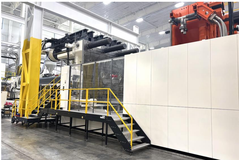
A view of the clamp area reveals the sheer size of the overall machine at 96 feet. (Picture: ENGEL)
