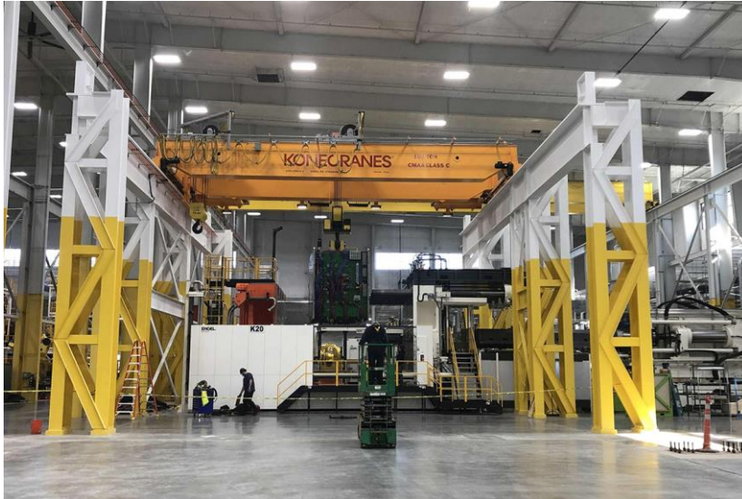
One of several large molds that can be installed in ENGEL 8200 ton clamp injection molding machine using a 150-ton crane. (Picture: ENGEL)
