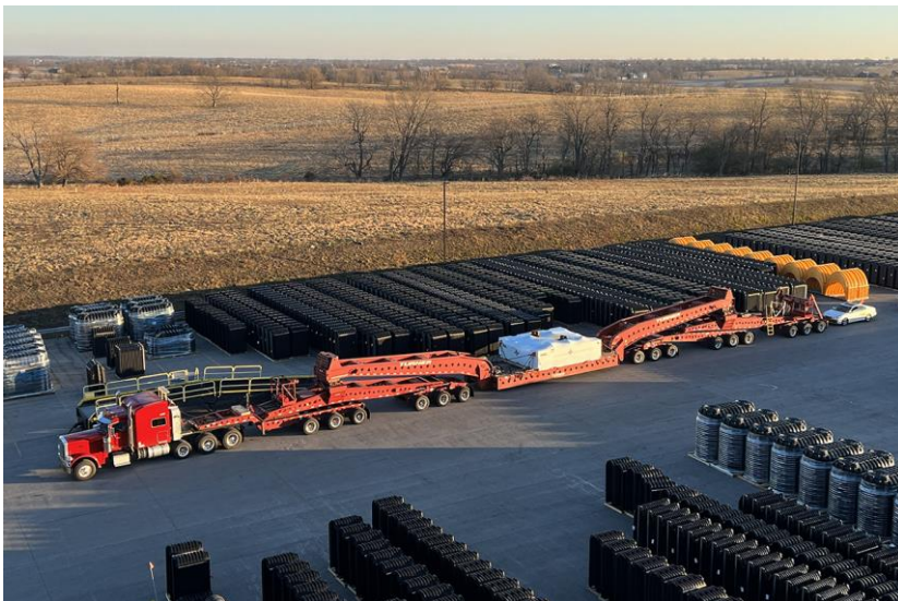
Special transportation was required for many parts of this huge machine. Pictured is the arrival of the 257,941 pound stationary platen at the Infiltrator facility in Winchester, KY. (Picture: ENGEL)
