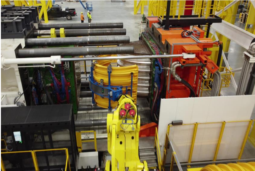
A seamless installation of automation for the handling of large parts with shot weights up to 270 pounds. (Picture: ENGEL)
