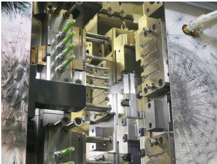
Servo-electric moulds are in greater demand, especially in medical technology. Digitalisation of the production processes is one driver of this trend. (Image: ENGEL)
