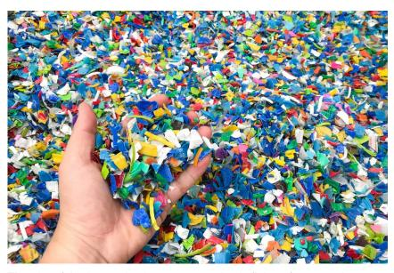
The aim of the innovation is to process plastic flakes, for example, from post-consumer collection, directly in injection moulding without pelletising.
