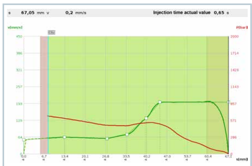
Fig. 2. The graphic display in the CC300 shows all the important information at a glance. The injection profile is displayed from right to left, corresponding to the direction of movement of the screw. The green lines represent the speed curves and the red line, the pressure curve (© Engel)
