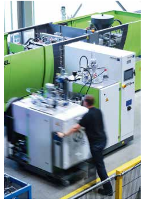
Fig. 4. The Multi-Connect color modules are designed as mobile carriages that dock on to the isocyanate unit and are controlled by it
