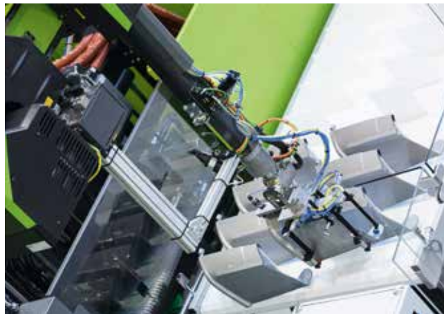
Fig. 1. The D-pillars were produced during Fakuma 2017 on a Duo injection molding machine (© Engel)
