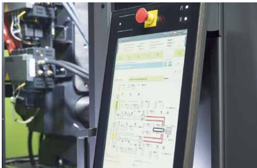
Fig. 3. The CC300 controller of the injection molding machine controls the entire process, including PU processing (© Engel)
