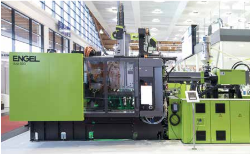
Fig. 1. The D-pillars were produced during Fakuma 2017 on a Duo injection molding machine (© Engel)
