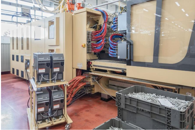
Temperature control on a small footprint. The number of cavities was increased, but the number of temperature control devices was reduced.
