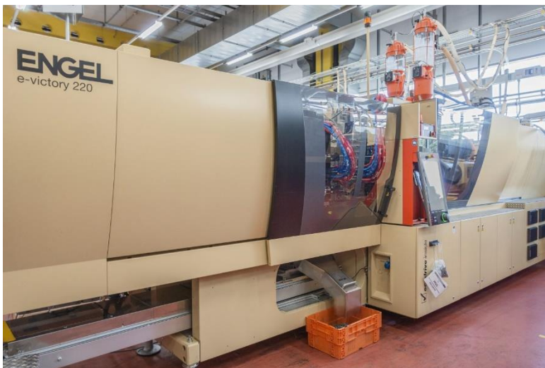
The e-victory 220 injection moulding machine is exclusively reserved for the production of damping cylinder housings.
