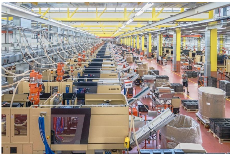
Tie-bar-less e-victory and victory machines make up the lion's share at the Blum plant.
