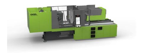
More mould space, smaller footprint: The new electric ENGEL victory electric 220 with 2200 kN clamping force enables compact production thanks to its tie-bar-less design and reduced machine length.
