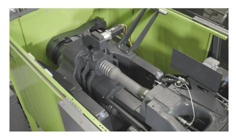
High energy efficiency, uniform force distribution and maximum repeatability: The new clamping system with pressure pad and ball screw ensures precise mould centring and shorter cycle times.
