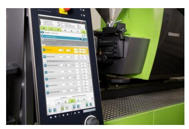
The new Parameter Limits feature makes it possible to define fixed tolerance ranges for up to 150 process parameters directly on the machine control unit.
