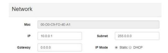
After the network settings have been modified successfully, connect the IoT device to your company network by means of an RJ-45 network cable.
