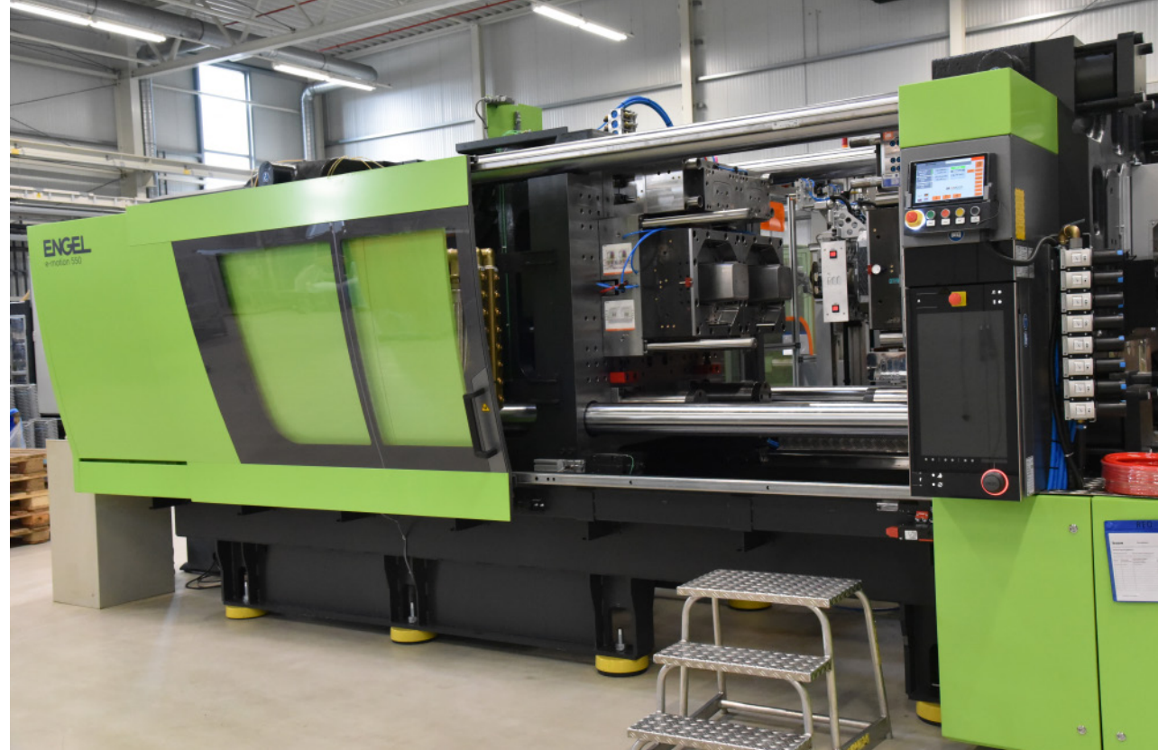
The ENGEL e-motion 550 at Ilsen accommodates moulds with a total weight of up to 7.3 tonnes.
