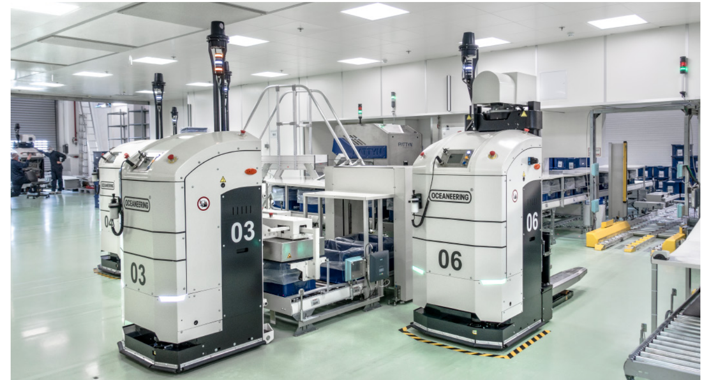
All logistical processes are performed by robots and driverless transport systems. The high-bay warehouse is connected to the 20,000-square-metre cleanroom.
