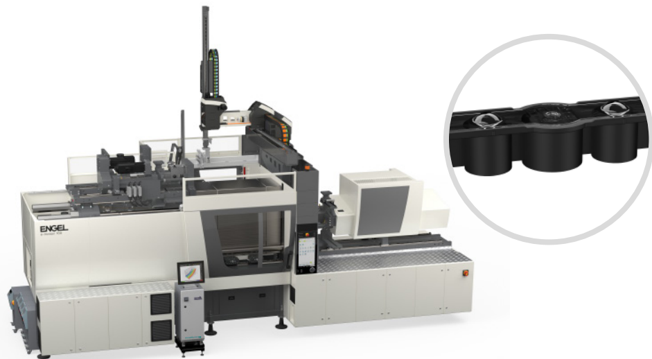
Extremely compact: combi M technology reduces the production cell's footprint. Under cleanroom conditions, ENGEL is moulding two-component sample vessels for medical diagnostics at its stand at K 2022.
