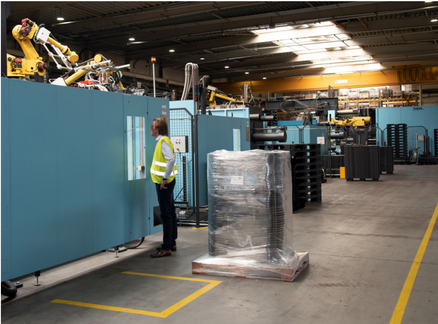
Comparing sizes: The new ENGEL duo 2300 with the two-stage process is several metres shorter than a conventional model from the same series right at the end of the production floor. This is also an important purchasing criterion for AVK.
