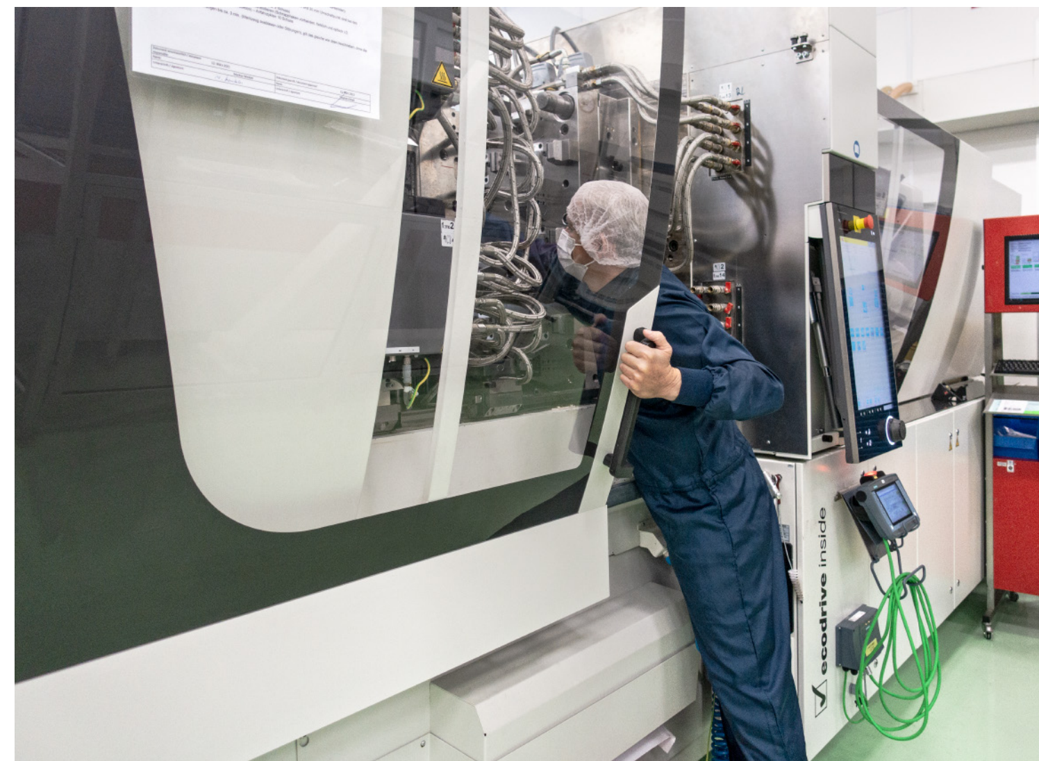
Barrier-free access to the clamping unit makes manual work on the mould particularly simple.
