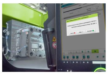
The optimum holding pressure time is often lower than the holding pressure time set initially. In these cases, the cycle time is reduced.
