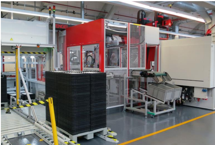
The robot transfers the housing parts from the mold directly to the quality control system, which is located on the rear of the injection molding machine.
