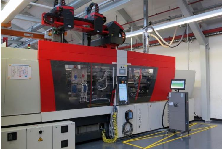
A tie-bar-less victory injection molding machine with an integrated viper 60 dual robot forms the heart of the production cell.
