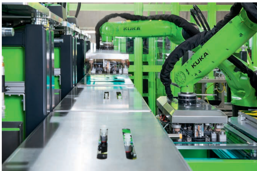
Fig. 5. The ready-cut tapes are separated at the stacking magazines and held in position on pick tables for collection by the robots © Engel
