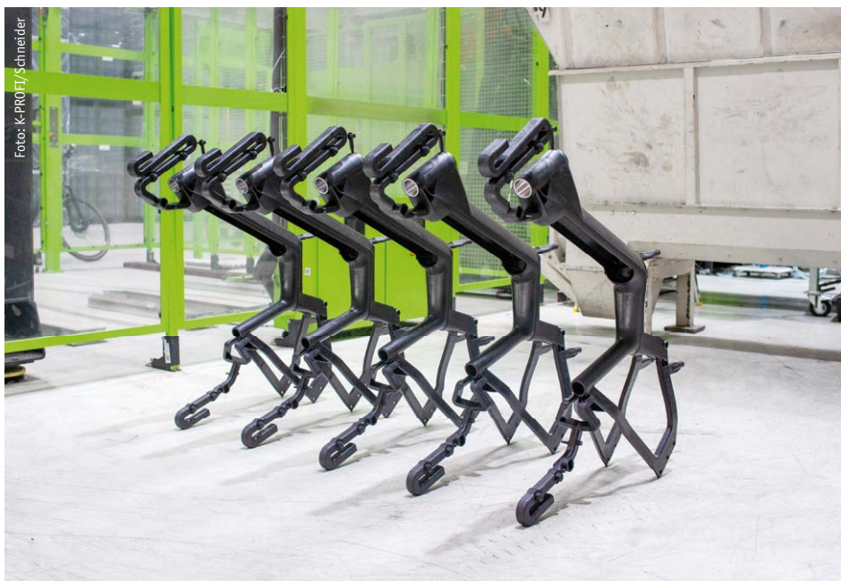
Freshly demoulded frames, still with the secondary cavities filled by the fluid injection technique.
