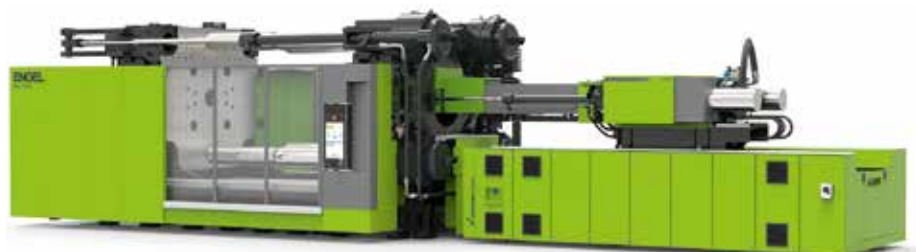
Fig. 5. The new injection units enable the hydraulic injection molding machines Victory and Duo (shown in the picture) to be selectively adapted to the users' individual requirements (© Engel)
