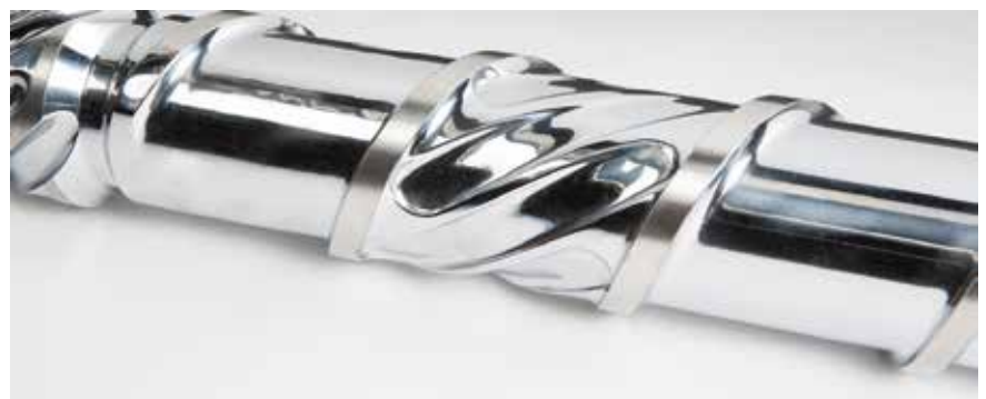
Fig. 2. The new screws obtain even greater performance boosts. The UAS (Universal Automotive Screw) increases the performance for processing a wide spectrum of materials, from PP, through glass-fiber-reinforced PA to shear-sensitive PC+ABS (© Engel)
