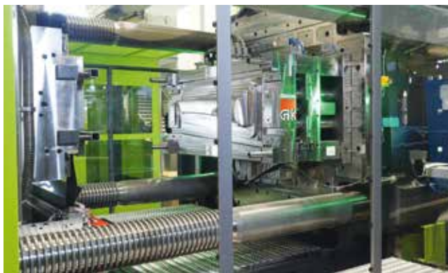
Fig. 2. Looking into the mold: in-mold graining gives the film the desired surface structure
