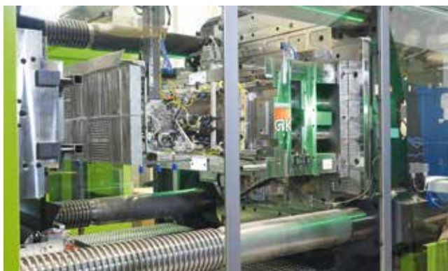
Fig. 3. The infrared heaters for heating up the film are integrated into the linear robot's grippers (© Engel)
