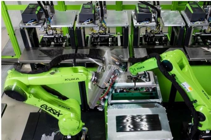
The integrated production cell delivers tailor-made composite blanks in one-minute intervals.
