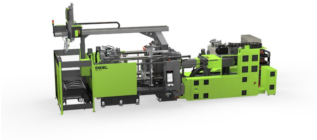
Image 1: Functionalised rear-end-lights are produced on the ENGEL duo 700 – with high precision and using clearmelt and foilmelt in a single integrated process with a compact footprint.
