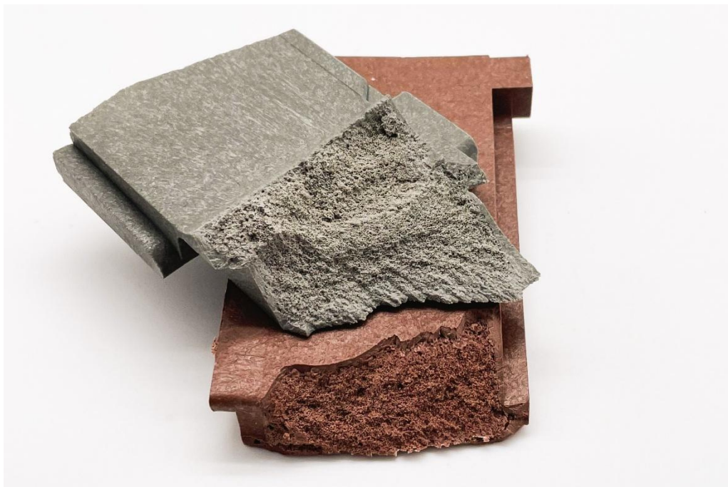
Image 2: Lightweight, stable, sustainable: Cross-section of the perfectly foamed component made from 100 percent post-consumer recyclate, delivering 30 percent less weight and 10 percent higher impact resistance.
