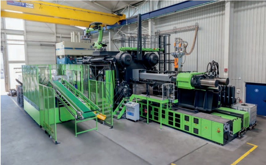
Fig. 3. The tests were carried out in the Schneider Form pilot plant on an Engel duo 23050/4000 injection molding machine (© Schneider Form)
