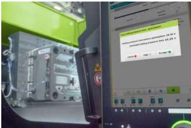
The new iQ hold control assistance system determines optimum holding pressure times, thereby enhancing efficiency in both setup and production operations.
