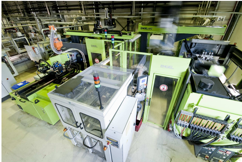
The manufacturing cell comprises two injection moulding machines, two linear robots and one multi-axis robot. (Picture: Helvoet)
