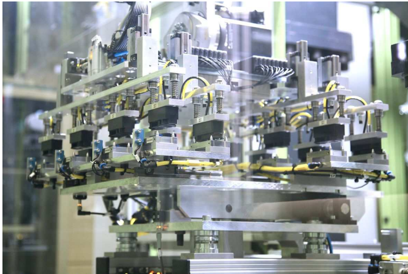
The gripper head is centred in the mould prior to the transfer of pre-moulded parts. (Picture: ENGEL)
