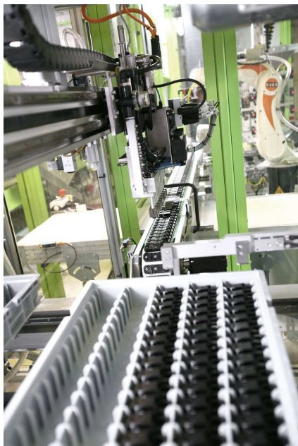
The multi-axis robot removes test cassettes from the mould and places them in trays for subsequent assembly and packaging. (Picture: ENGEL)
