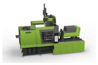
Featuring smart assistance software, the all-electric e-mac injection moulding machine automatically compensates for fluctuations in the raw material to ensure consistently high part quality.
