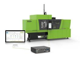
The new iQ process observer analyses several hundred process parameters across all phases of the injection moulding process and points out counterproductive process settings and conditions.
