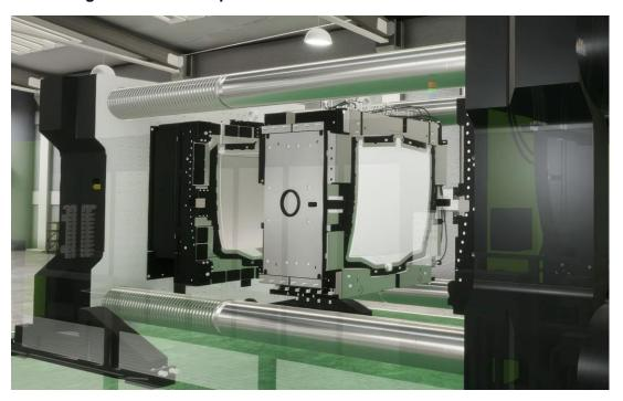
'In-mould coating' eliminates the need for expensive downstream painting lines: PUR flooding in the ENGEL clearmelt process.
