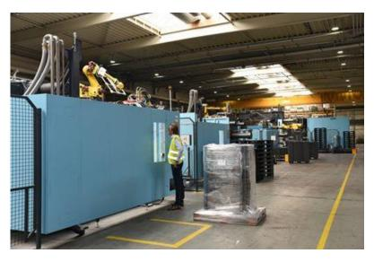
Comparing sizes: The new ENGEL duo 2300 with the two-stage process is several metres shorter than an older machine from the same model series right at the end of the production floor. This is also an important purchasing criterion for AVK.
