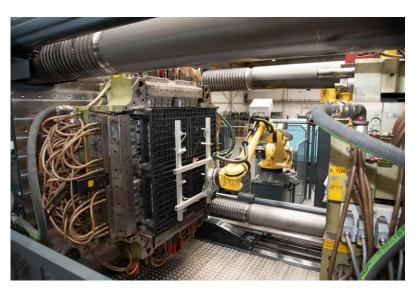
ENGEL duo 1500: 28 kilogram shot weight. Plasticising takes place continuously during the cycle, while the cavity is fed by a piston unit. The pallets are taken off and deposited automatically.
