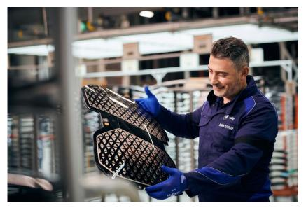
The kidney-shaped badges for the new BMW iX are produced in a highly integrated cleanroom production cell by ENGEL. This is the first series production application for combined film back injection moulding and polyurethane flooding on the demanding vehicle exterior.
