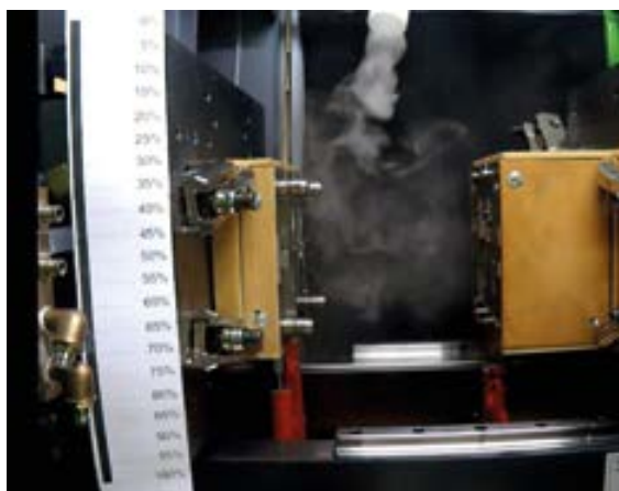
A constant airflow no longer prevails at a mould temperature of 90°C.
