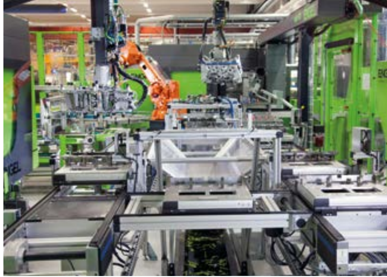
The circulating conveyor system at the centre of the production cell links the three victory 120 machines that produce the knife hilts.
