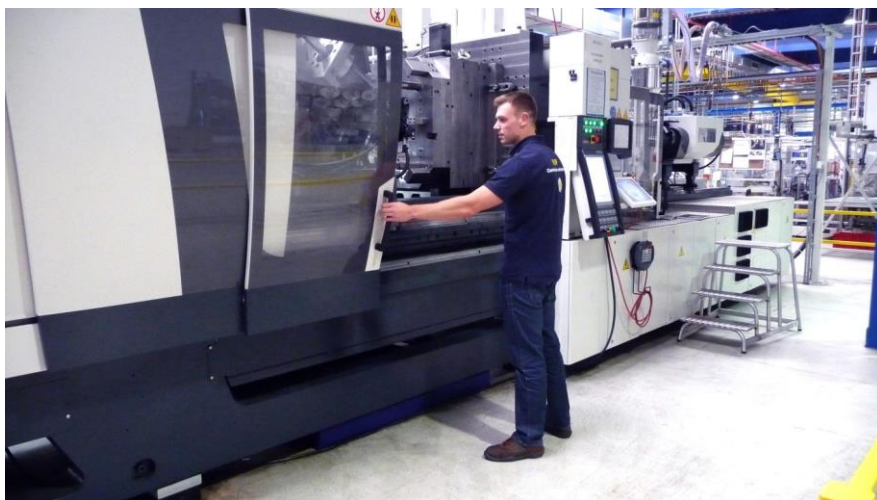
In its new design the ENGEL victory 500 injection moulding machine features a two-part safety gate.
